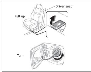
**NOTE:** If the cap is not tightened enough, Check Engine " $\bigotimes_{i=1}^{\infty}$ " indicator may illuminate.
